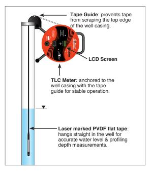
A Tape Guide/Datum allows the depth measurement to be read at the marked position on the Tape Guide, to give reliable, repeatable, accurate depth measurements when profiling a well. The Tape Guide protects the tape from damage on rough edges of well casing.
